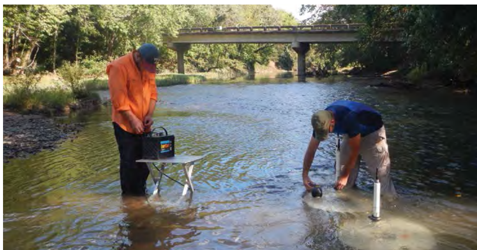
Sediment oxygen demand chambers deployed in 2017 measure the oxygen consumed by micro-organisms in the river's sediments.
